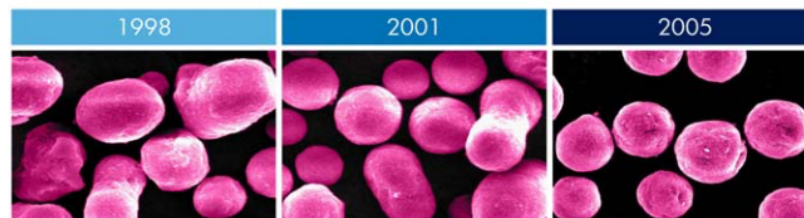
Figure 4. Improvements over time have made new HP ColorSphere toner more uniform in particle size, size distribution and shape. Toner charges faster, enables faster fusing, and maintains its charge throughout the life of the cartridge.
